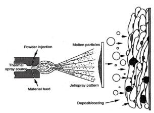
Figure 1. Schematic representation of the thermal spray process flow and layer build-up
