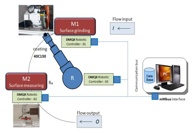
Figure 9. The flexible robotic cell for grinding process optimization
