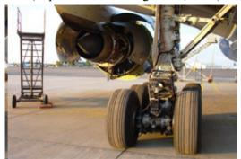
Figure 2. Thermal spray coated landing gear struts -replace hard chromium plating
