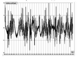
grinded surface roughness profile (b.) Figure 4. Measuring surface roughness with RUGOMAS instrument
