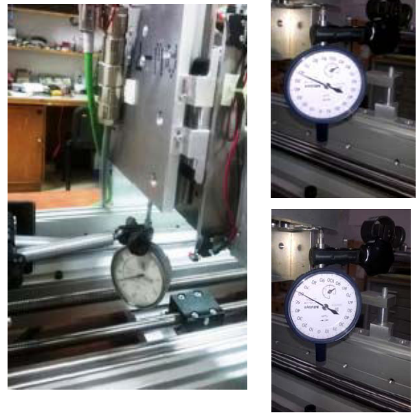
Fig. 14. Checking repeatability positioning accuracy
