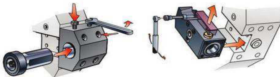
conversia unei turele standard la sistem Coromant Capto
