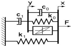
Fig. 3. Bouc-Wen modified mechanical model
