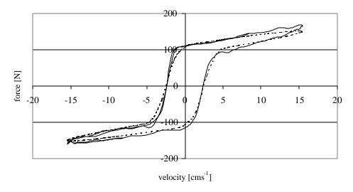
Fig. 4b. Force vs. velocity for 0.06 A \_\_\_\_\_ experimental; ..... predicted
