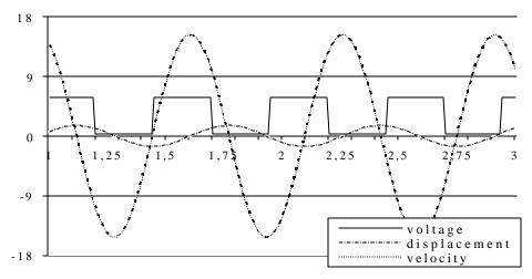
Fig. 9a. Time histories of the voltage [volts], displacement [cm] and velocity [cm/s] in the first test case
