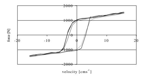
Fig. 5b. Force vs. velocity for 1.75 A \_\_\_\_\_ experimental; ..... predicted
