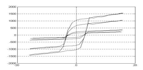
Fig. 2. Force [N] vs. velocity [cm/s]
