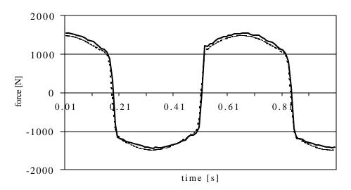
Fig. 5a. Force vs. time for 1.75 A \_\_\_\_\_ experimental; ...... predicted
