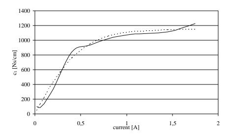
Fig. 7. The parameter  $c_1$  vs. current u, experimental ( \_\_\_\_) and predicted (....)
