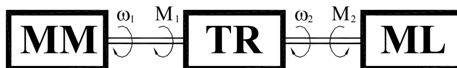
Fig. 1 – The scheme of the drive system.
