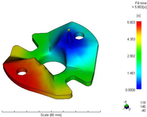
Fig. 3 – Mold filling diagram.
