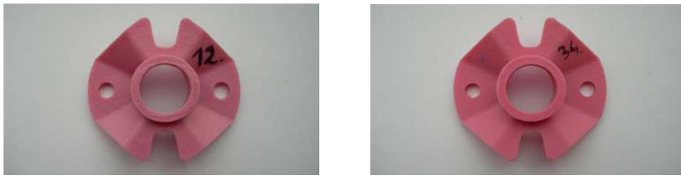
Fig. 8 – Example of 863 Pink molded part (6 vents, mold temperature –50°C, filling time of mold cavity –5.8 s).
