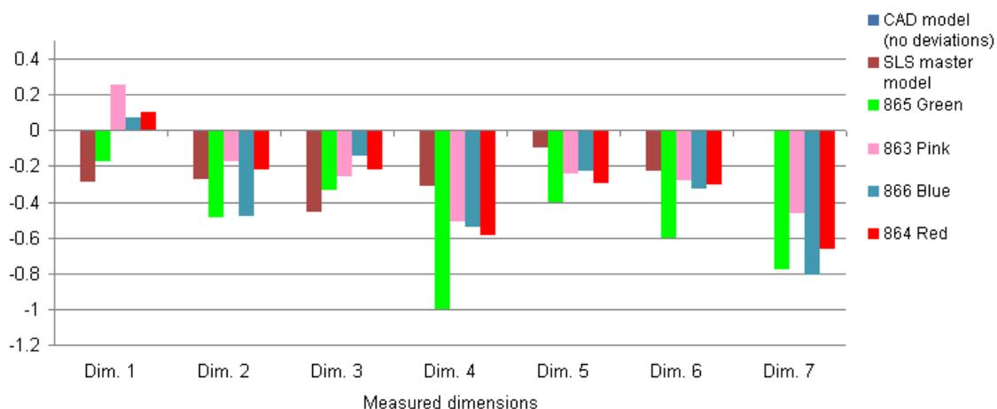
Fig. 10 – Deviations of wax part dimensions related to CAD model and SLS master model.
