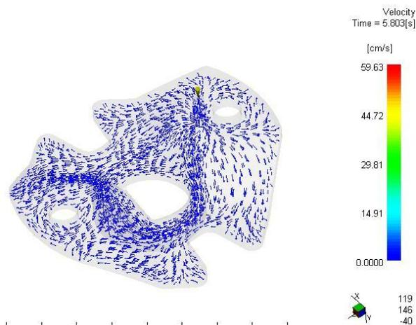
Fig. 5 – Movement of the wax molecules in mold cavity.
