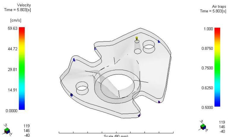
Fig. 6 – View of air traps positions.
