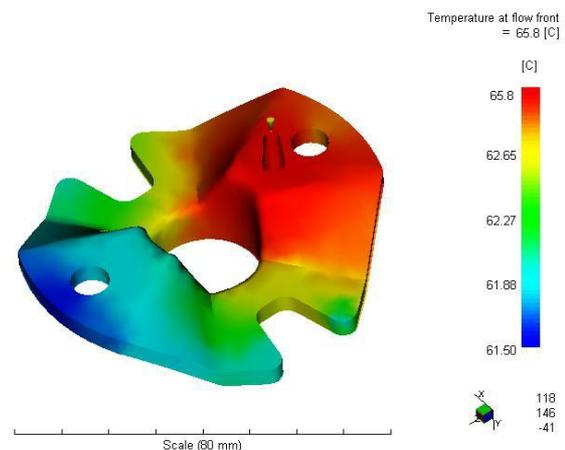
Fig. 2 – Temperature evolution in vacuum casting of wax.
