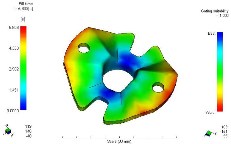
Fig. 4 – Optimal casting points.
