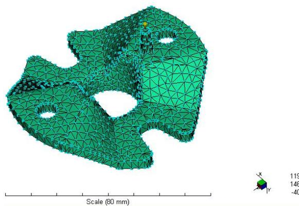
Fig. 1 – Finite elements network obtained from meshing and casting funnel placement.
