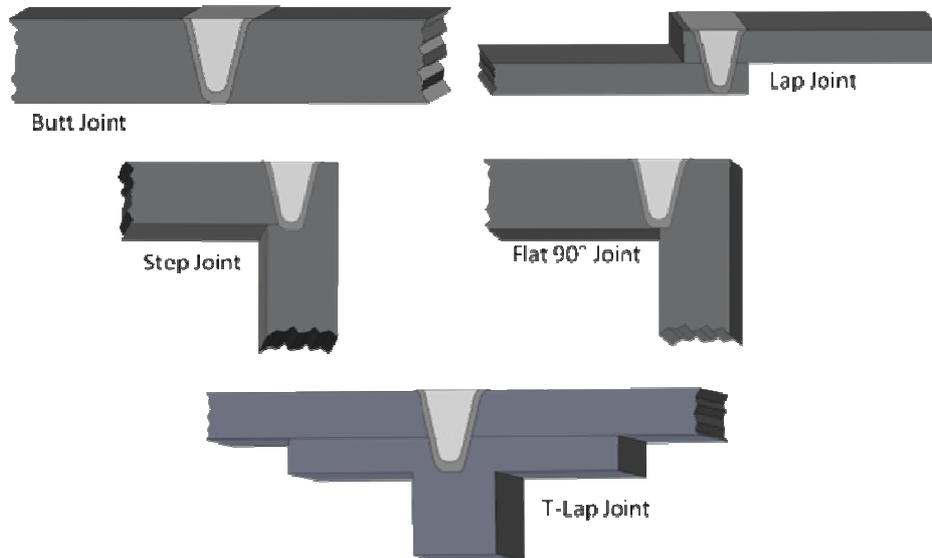
Fig. 2 – Joint configurations for FSW.
