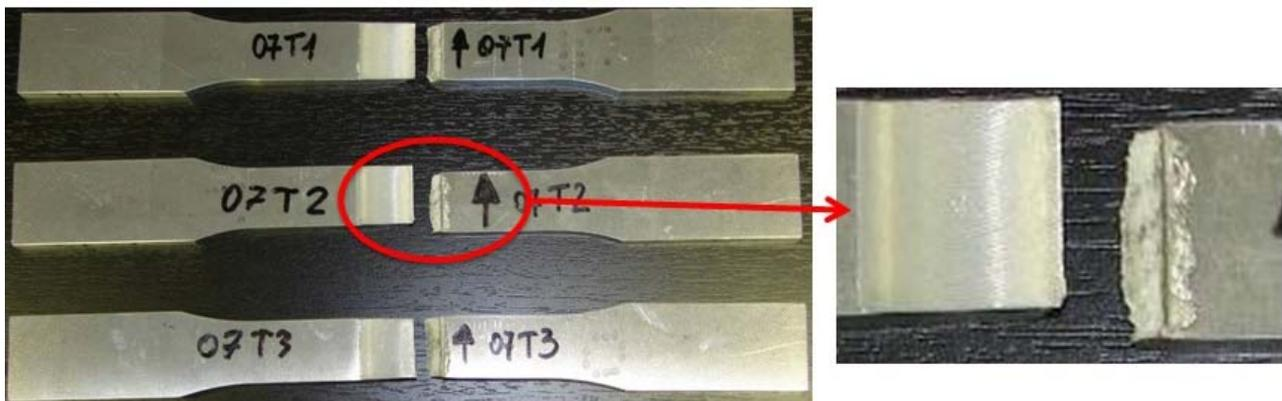
Fig. 11 – Tensile specimens breakage.
