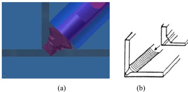
Fig. 3 – a) Welding tool for fillet connections; b) fillet joint.
