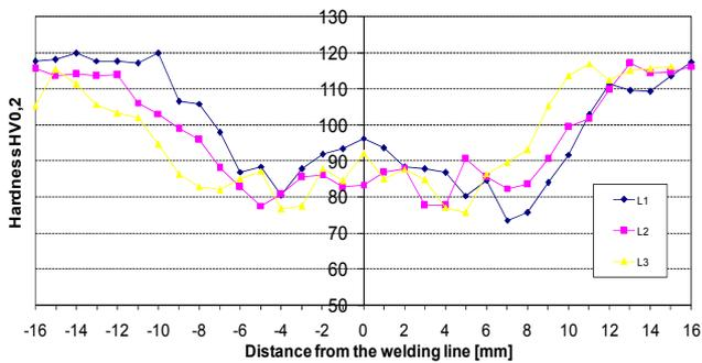
Fig. 9 – Hardness measurements on AA 6082-T651.
