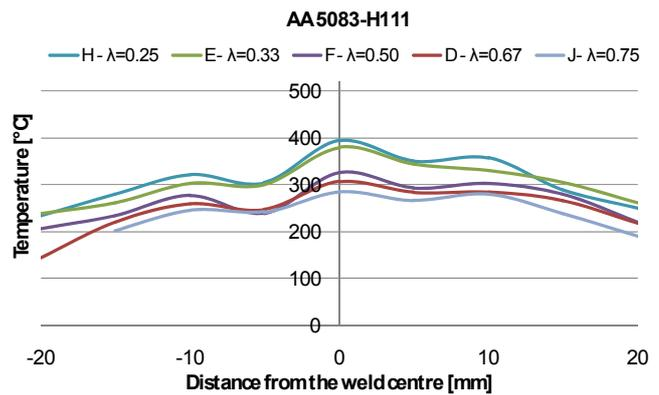
Fig. 6 – Temperature measurements on AA 5083-H111.
