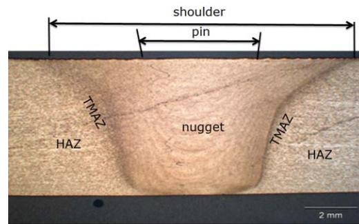
Fig. 8 – Macrostructure analysis on AA 5083-H111.
