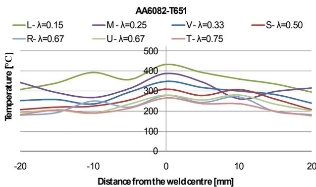
Fig. 5 – Temperature measurements on AA 6082-T651.
