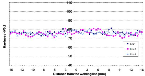
Fig. 10 – Hardness measurements on AA 5083-H111.
