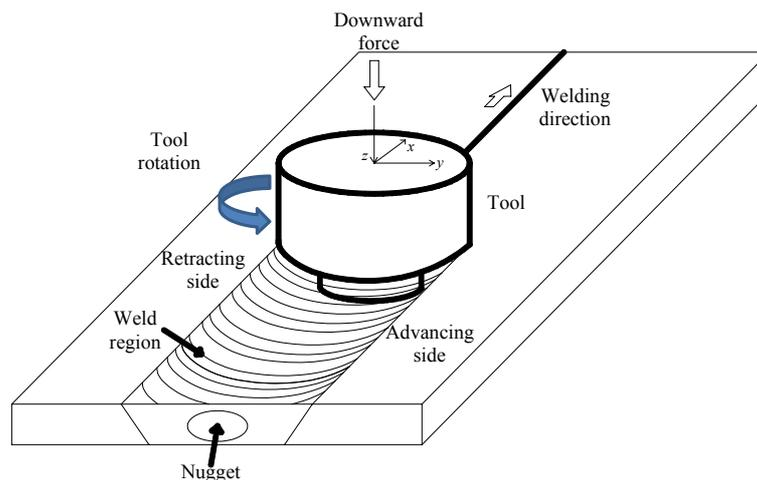
Fig. 1 – Schematic of the friction stir welding process.
