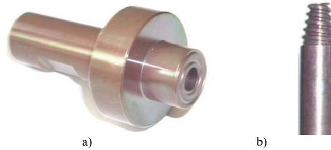
Fig. 4 – Welding tool: a) flat shoulder with machined spiral flute, 15 mm diameter; b) threaded pin with thread M6L, conical tapered with three milled flats, 5 mm diameter.
