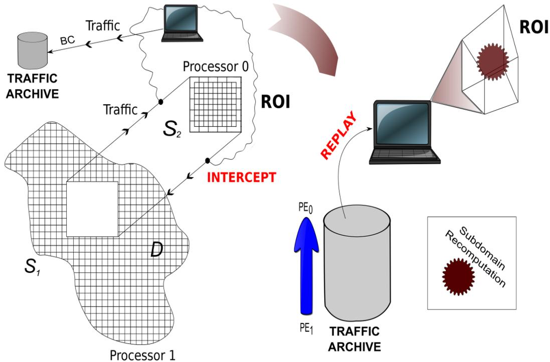
Fig. 2 – Traffic interception and later replay during the reconstruction of the fields.
