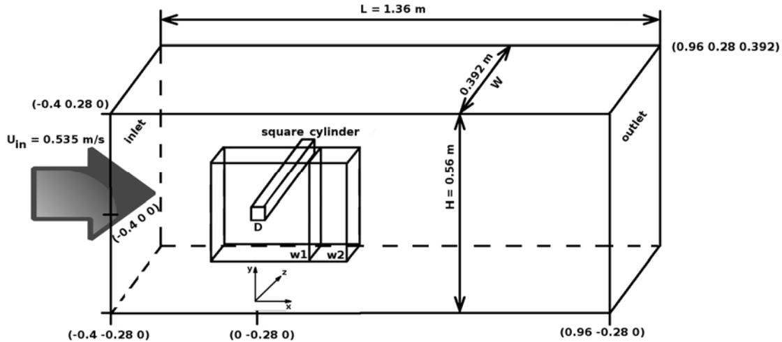
Fig. 4 – Computational domain and boundary conditions (BCs).
