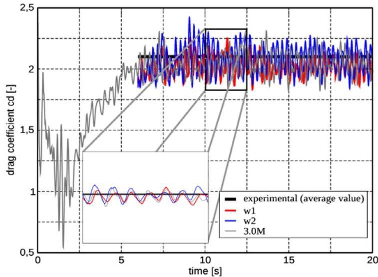
Fig. 5 – Validation of the numerical results against experimental data.
