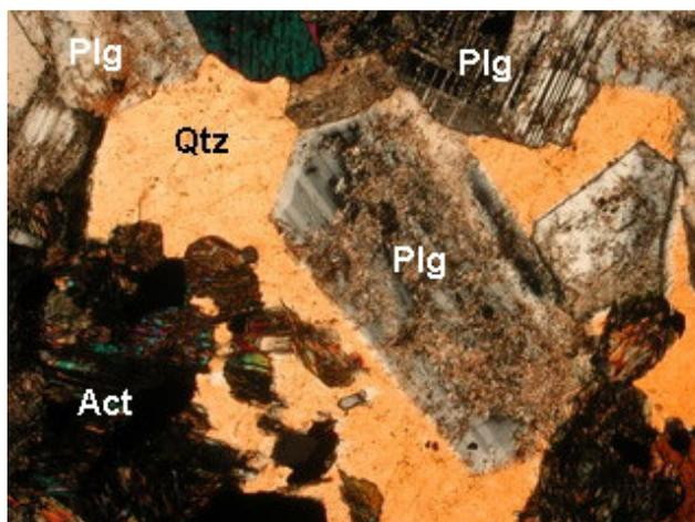
Fig. 6. Twinned euhedral plagioclase with albite rim, partially sericitized, included in anhedral quartz and pseudomorph of fibrous actinolite (uralite) after older pyroxene (N+ 40×).
