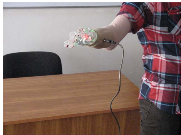
Figure 4. Patient using a prototype of the bionic hand, in training.
