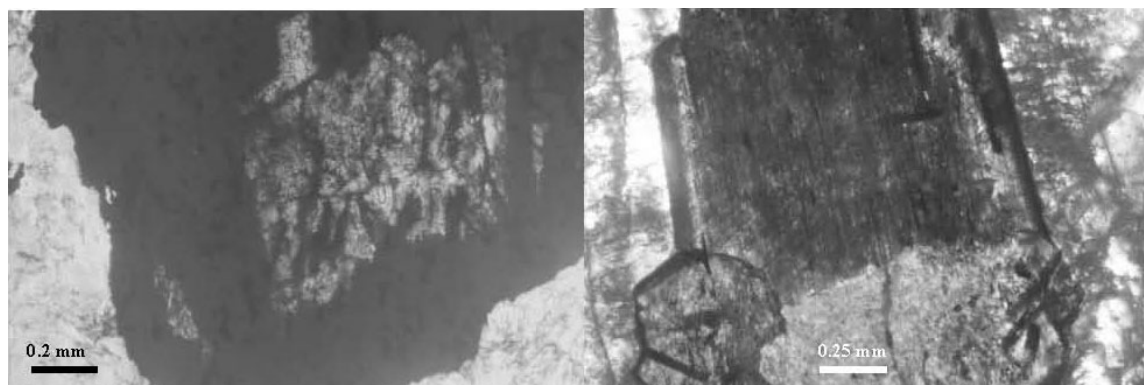
Fig 12. Nb-rutile (brownish yellow) substituted/intergrowth by/with niobian Mn-ilmenite (black), sample Dt2006/13 (left); unmixed Mn-ilmenite (?) (brown) in niobian rutile (greenish yellow), sampleBel/13A (right photo).
